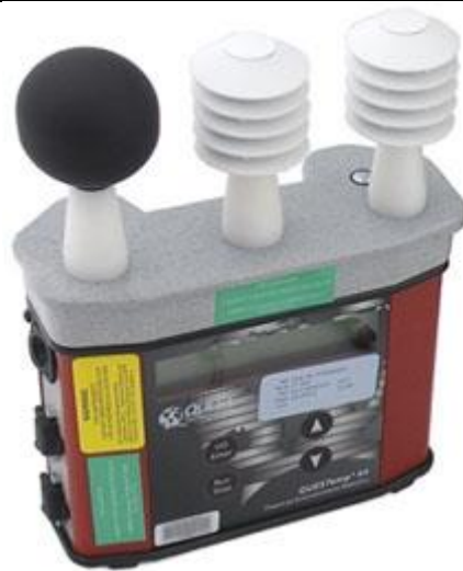
Figure 3: Waterless wet-bulb meter
