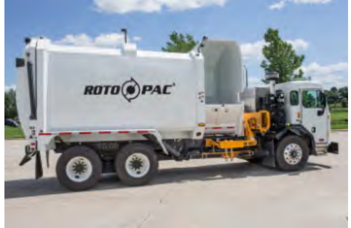
Figure 3.8 ROTO PAC Organic Waste Collection Truck with Auger Packing System
