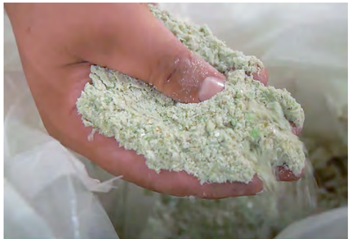
Figure 3.11 Glass Crushed to Sand (Courtesy Aqua Tools)
